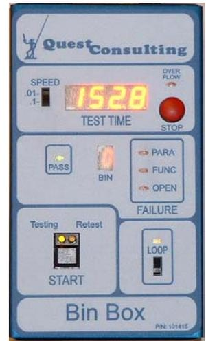
The Bin Box also has a 4-Digit counter that displays the Test Time from the **Start Test** signal to the **End-of-Test** signal. At the “End-of-Test” the counter stops and displays the total test time.
