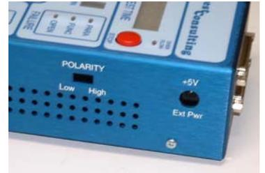
The Polarity slide switch is easily accessed via a small slot located on the right side of the Bin Box. To change to active LOW or active HIGH, slide the switch to the position as labeled.
