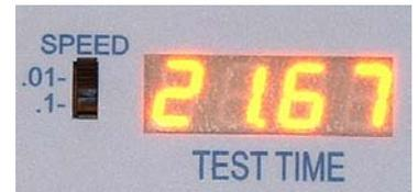
**Test Time Counter:** The four-digit display shows the time (in tenths or hundreds of a second) the tester has spent on a test. Counter stops running at End-of-Test.
