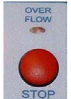
**Stop Push Button:** Halts the Test Time display (but does not stop the present test). Will also take Bin Box out of Loop Mode.
