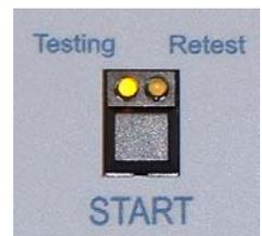
**Testing LED:** Yellow LED turns on when a test is in progress.
